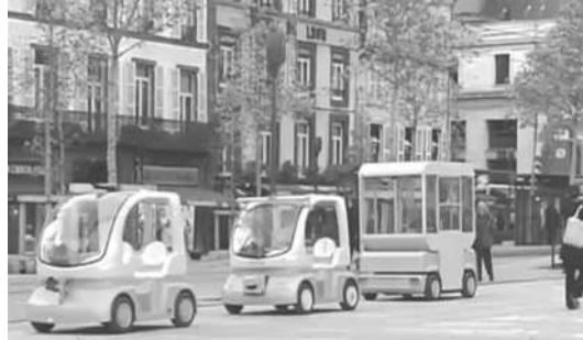
FIGURE 6.4 (See color insert) Example of autonomous navigation in formation of a group of UGVs in an urban environment (Clermont-Ferrand, France). MobiVIP project (Predit 3).
