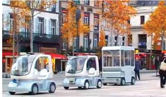
COLOR FIGURE 6.4 Example of autonomous navigation in formation of a group of UGVs in an urban environment (Clermont-Ferrand, France). Mo-biVIP project (Predit 3).
