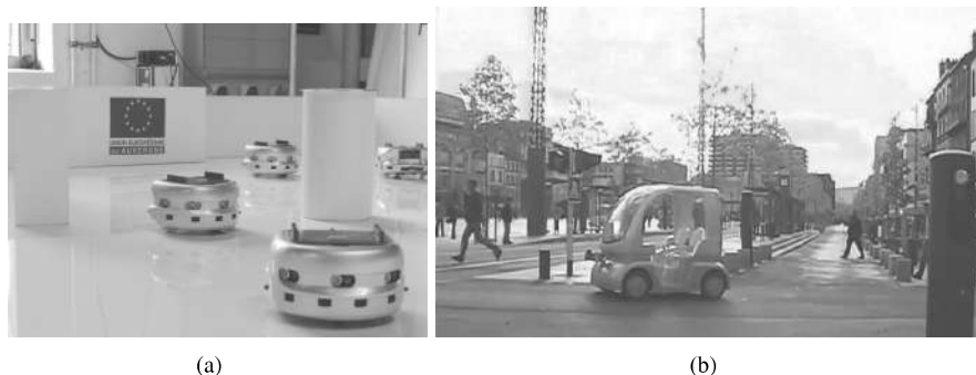
FIGURE 2.1 (See color insert) Autonomous navigation of (a) a group of mobile robots (Khepera ® ) and (b) an electric vehicle (Cycab ® ) in an urban environment (Clermont-Ferrand, France). MobiVIP project (Predit 3).
