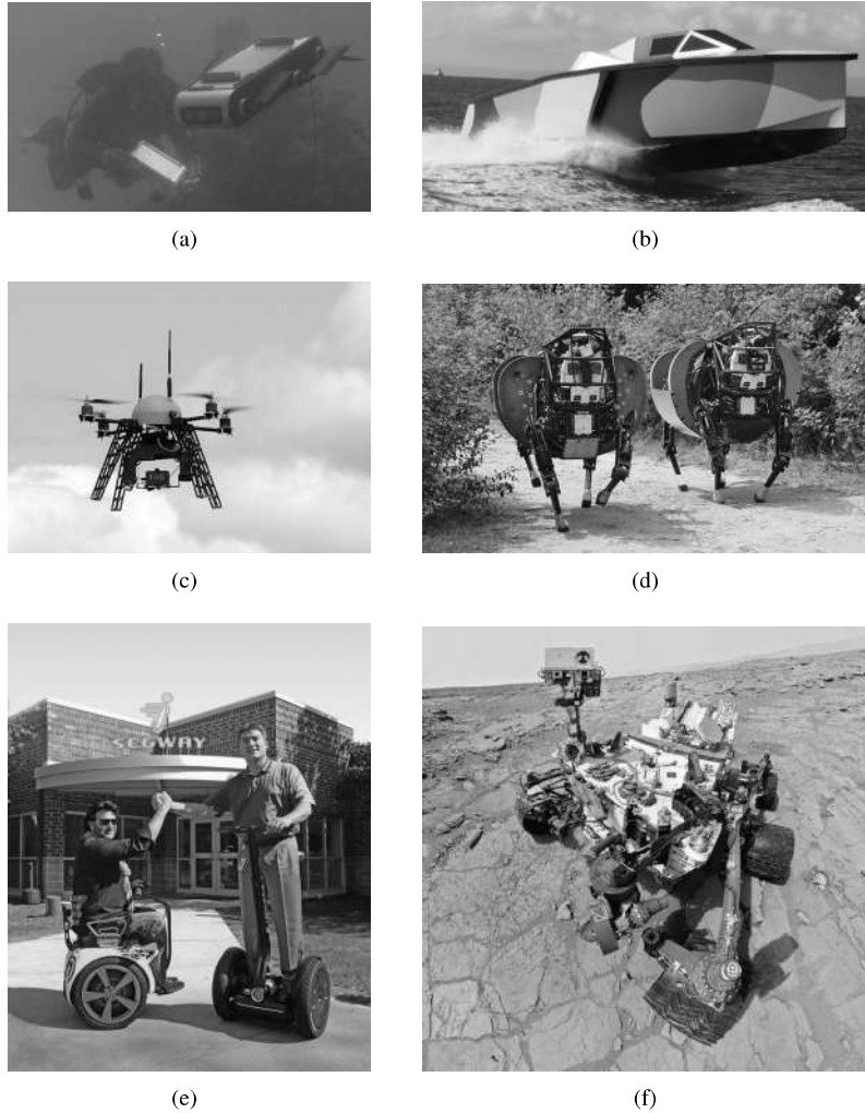
FIGURE 1.1 (See color insert) Different kinds of mobile robot locomotion. (a) AQUA ® bio-inspired AUV (KROY version) [Speers and Jenkin, 2013], (b) Piranha ® USV from Zyvex ® company, (c) UAV from Fly-n-Sense ® company, (d) two LS3s from Boston Dynamics ® , (e) the first two-wheel self-balancing chair Genny ® , inspired by Segway ® , (f) Robot Curiosity (from NASA) exploring Mars planet.
