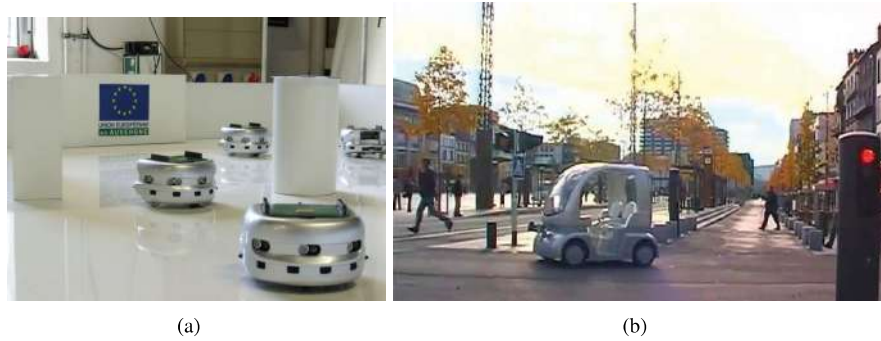
COLOR FIGURE 2.1 Autonomous navigation of (a) a group of mobile robots (Khepera ® ) and (b) an electric vehicle (Cycab ® ) in an urban environment (Clermont-Ferrand, France). MobiVIP project (Predit 3).
