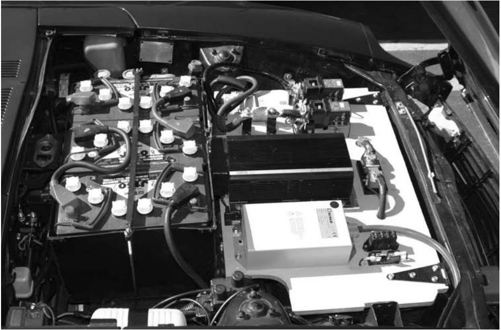
FIGURE 10-17 Operation Z battery mounted in place.
