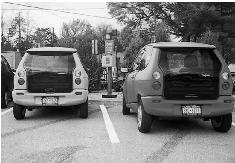
FIGURE 2 TH!NK City car s charging with A VCON charger s at Chappaqua train station. (Photo courtesy of Town of New Castle.)
