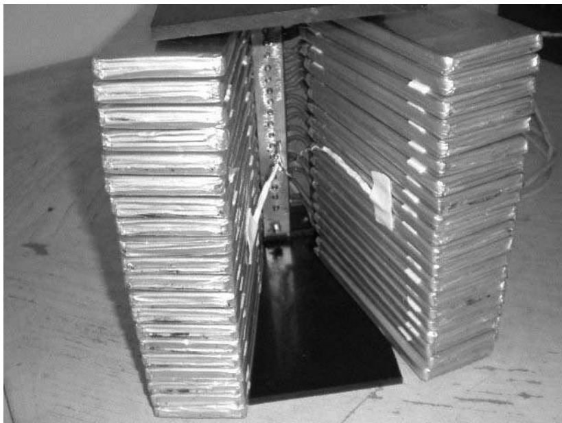
FIGURE 8-9 Lithium batteries ready to go into a Porsche for great speed and great range (Courtesy of EVPorsche.net).
