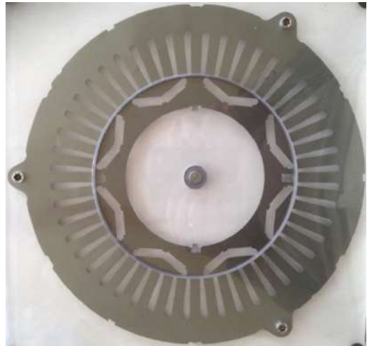
Figure 6.6 Views of the IPM rotor from the 2007 Toyota Camry HEV motor [1]. (Courtesy of Oak Ridge National Laboratory, US Dept. of Energy.)
