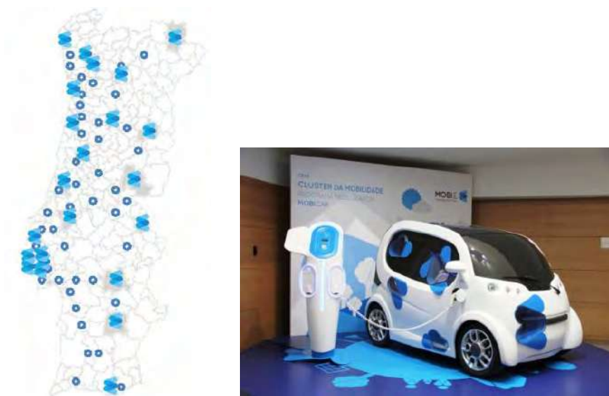
Fig. 24.5 MOBI.E vehicle electrification project includes installing charging stations in 25 municipalities and along main highways in its pilot phase (shown on the Portugal country map at left) as well as developing its own 80-km range battery-electric vehicle Mobicar, primarily aimed at the export market. (Source: MOBI.E.)
