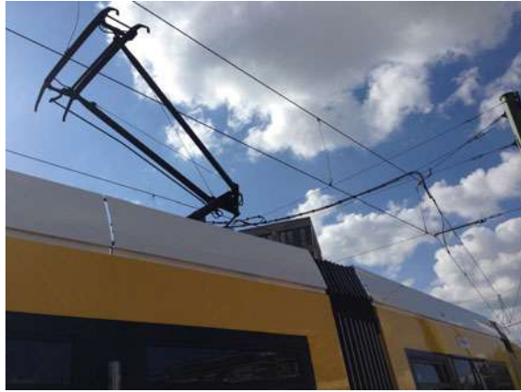
Fig. 2.5 Picture of a tramway's pantograph in contact with a catenary line. Source Author
