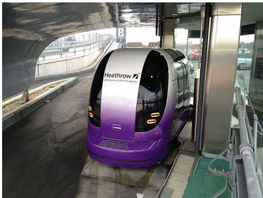
Fig. 2.15 Heathrow Airport car park operational PRT system. Source Picture of ULTra PRT POD at Heathrow Airport car park During a trip to the airport 2012-02-16; Author: Moshrunners; file is licensed under the Creative Commons Attribution-Share Alike 3.0 Unported license
