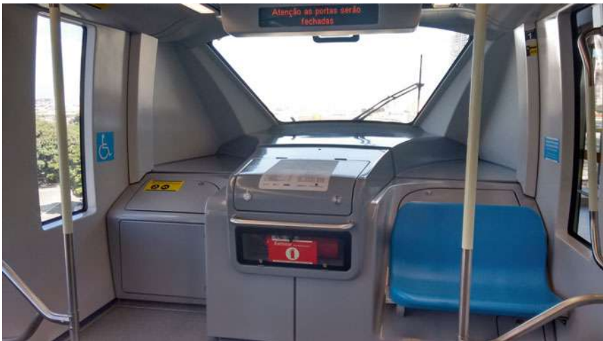
Fig. 2.9 A view of a monorail GOA 4 operation front end, without any driver or attendant in the city of Sao Paulo in Brazil. Source Author
