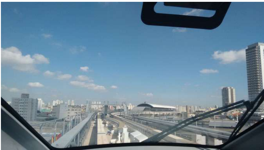
Fig. 2.7 View from a monorail's front car, showing heavy concrete switch beams managed automatically by a CBTC system. Source Author
