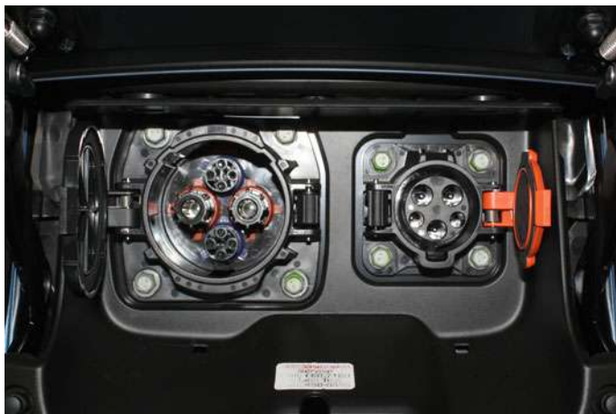
Fig. 3.7 Charging sockets on a 2012 Nissan Leaf TM . The socket on the left is a CHAdeMO connector for fast DC charging, and the socket on the right is an SAE J1772 connector for normal AC charging (Picture from Musashi1600 (Own work) [CC BY 3.0 us] ( http://creativecommons.org/licenses/by/3.0/us/deed.en ), Licensed under [CC BY 3.0 us]; via Wikimedia Commons)
