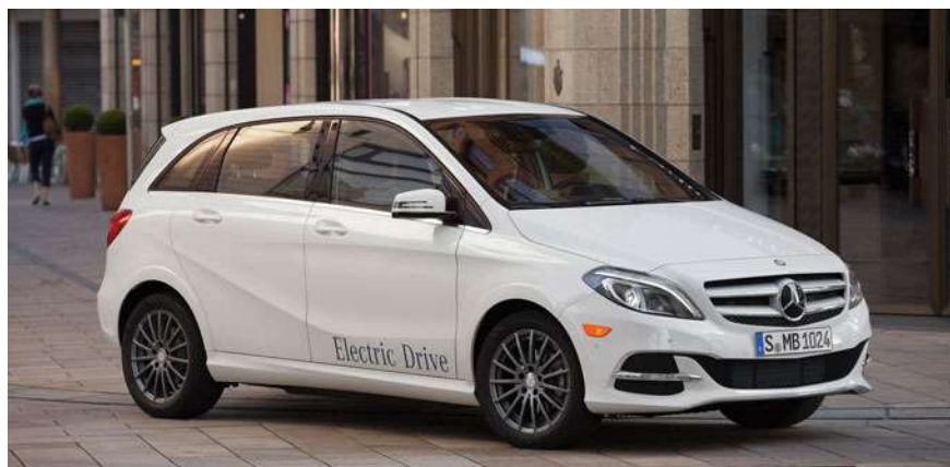
Fig. 3.2 The B-class electric drive from Mercedes Benz was rated by the EPA with a range of 140 km and an energy consumption of 25 kWh/100 kms for combined city/highway driving. Copyright of Mercedes Benz (Picture External view of the B-Class electric drive car, Copyright of Mercedes Benz and kindly lent for this book)
