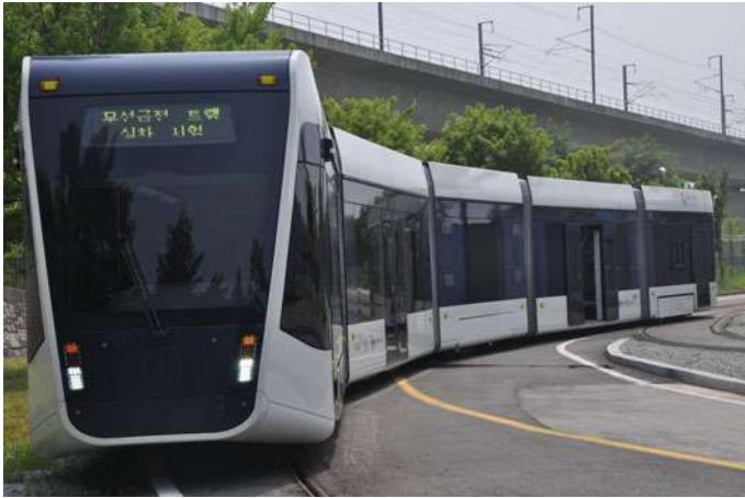
Fig. 2.5 SMFIR-based tram tested in Korea (90 kHz power supply)
