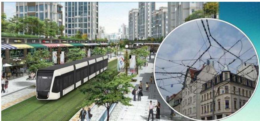
Fig. 17.4 Improved urban landscape by applying a wireless power transfer system to a low-floor tram
