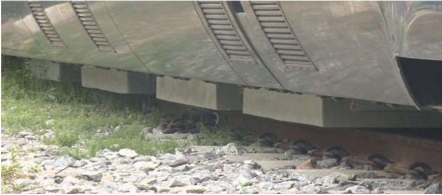
Fig. 17.11 Photograph of installed four pickup units
