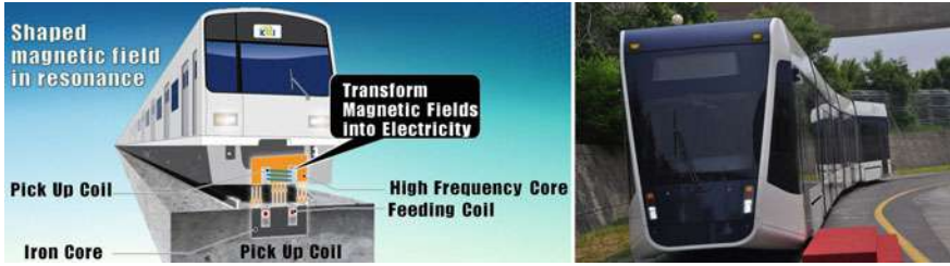
Fig. 17.1 Schematic diagram of a wireless power transfer system and its application to low-floor tram demonstration
